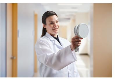
The proven technology, utilizing silicon diodes combined with an energy compensated Geiger-Müller tube, provides high sensitivity and stability over a very wide energy and dose rate range.
