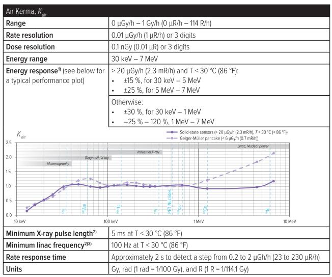
1. The instrument uses a Geiger-Müller pancake at low rates and a cluster of solid-state sensors at high rates. The rate where the solid-state sensors are fully engaged gradually increases with temperature, for temperatures above 30 °C (86 °F).
